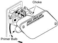
• Pull starter rope handle sharply 6 times. NOTE: The engine may sound as if it is trying to start before 6th pull. If so, go to the next step immediately.
